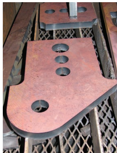
Producing laser-cut parts from plate allows Debro Steel to be competitive in a wide range of industries.
